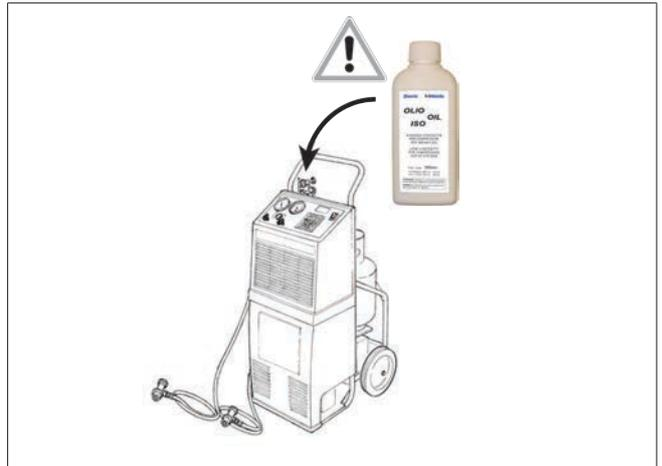
Fig. 25 Add the correct quantity of lubricant
