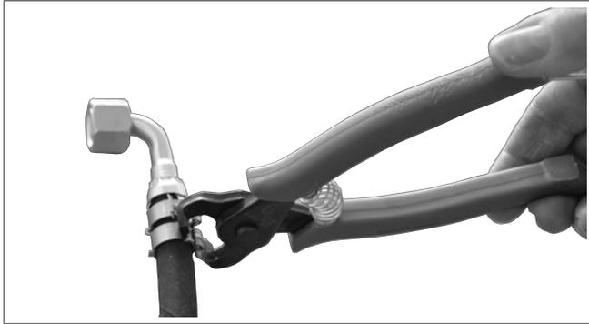
Fig. 12 Tighten the clamps
