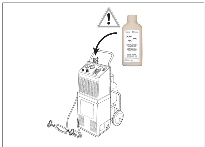
Fig. 7 Add the correct quantity of lubricant
