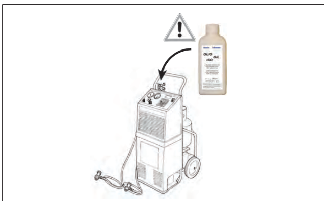
Fig. 16 Add the correct quantity of lubricant
