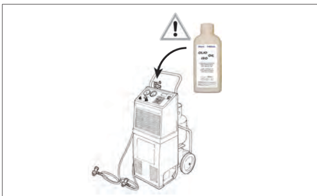
Fig. 16 Add the correct quantity of lubricant
